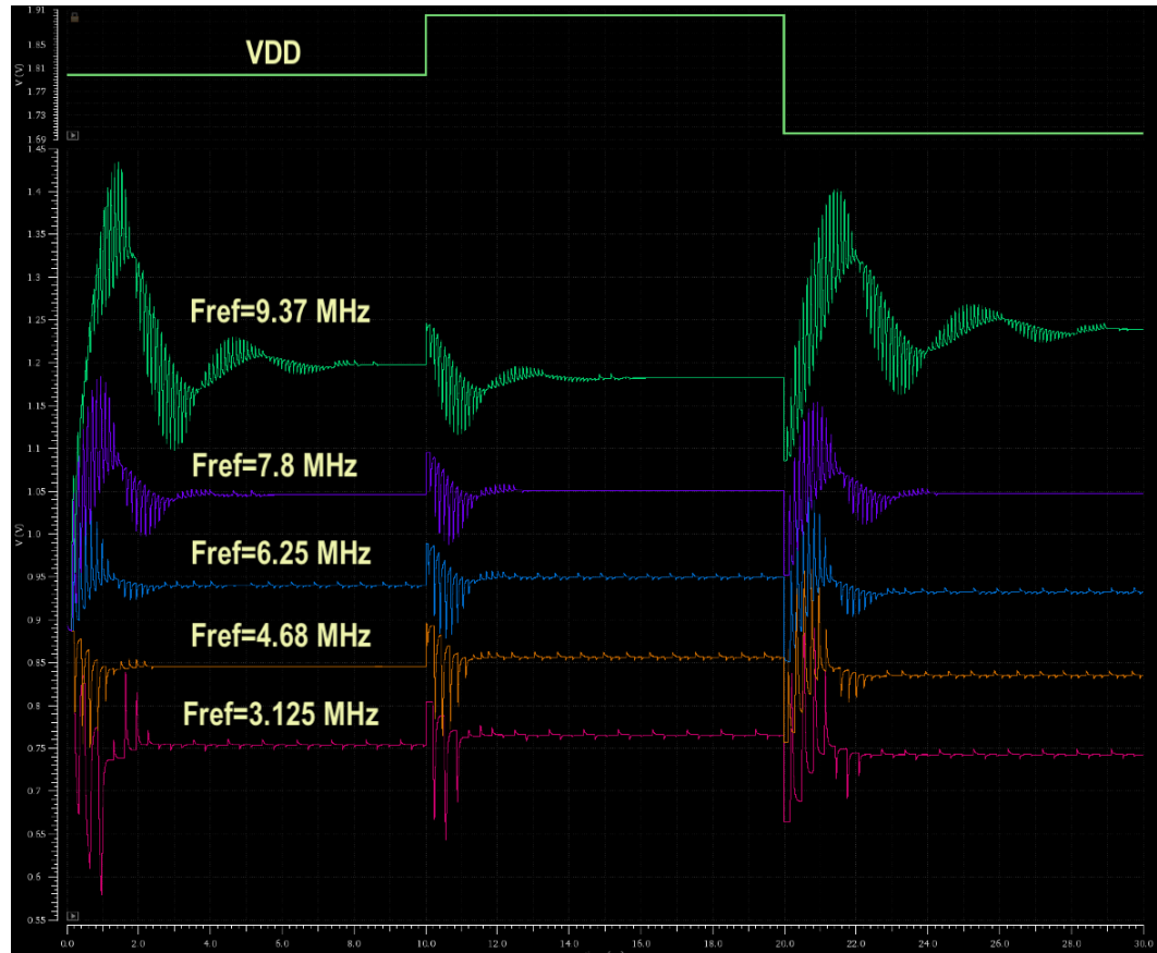
Figure 11: Input voltage of the VCO, test case 2.
